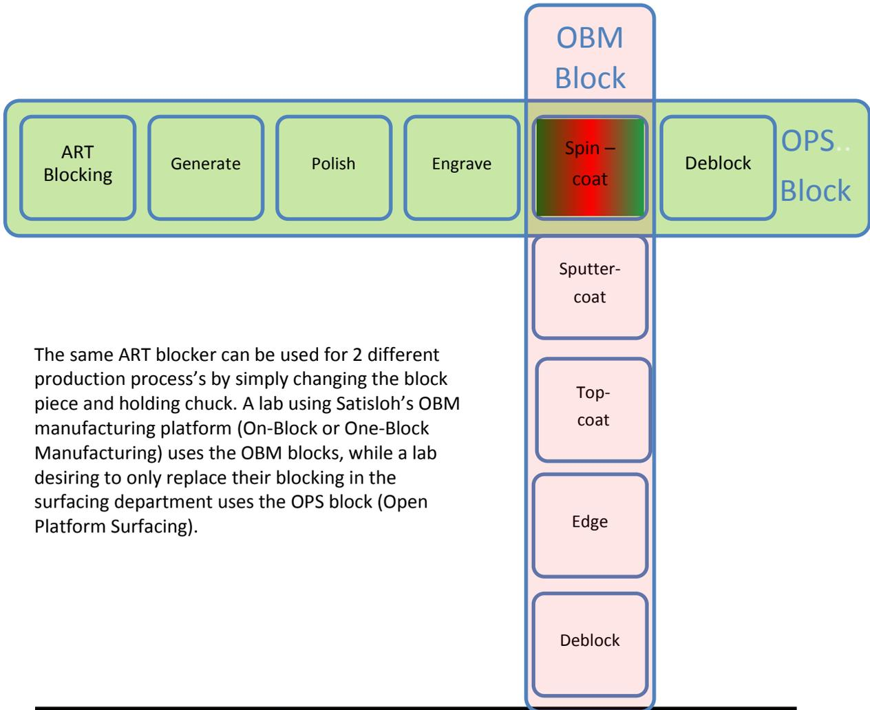
The same ART blocker can be used for 2 different production process's by simply changing the block piece and holding chuck. A lab using Satisloh's OBM manufacturing platform (On-Block or One-Block Manufacturing) uses the OBM blocks, while a lab desiring to only replace their blocking in the surfacing department uses the OPS block (Open Platform Surfacing).
