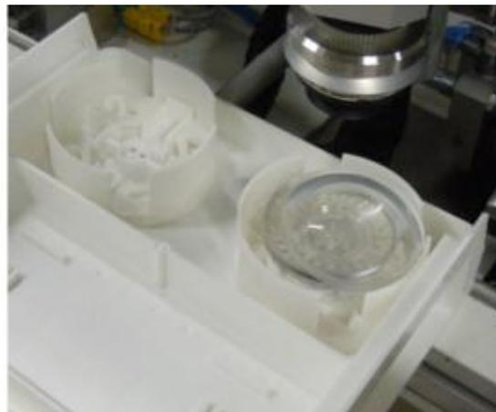
Picture 12: OPS Overlap (block smaller than lens)
