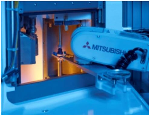
The next tray is put into position for the loading arm to pick the next lens to be measured by the LIS.
