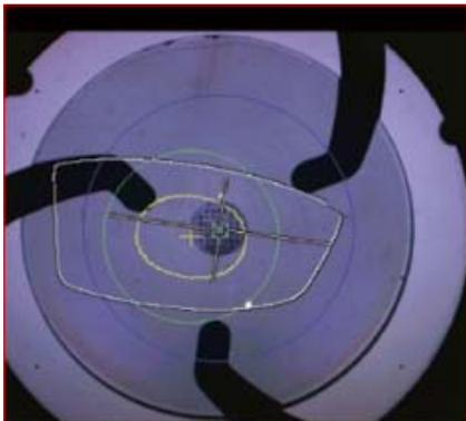
Progressive Addition Lenses (PAL) are easily detected by using engravings as reference points for measuring RX values as well as layout.
