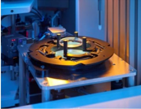
Once the edging cycle is completed the gripper picks up the lens. The lens is briefly tilted to remove any excess water residue. The loading arm rotates outside the edging chamber and loads the next lens into the clamping system. Once done the gripper drops the finished lens back into the job tray.
