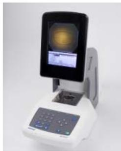
It can be a manual or automatic device. Layout and decentration are done at the blocker. Once blocked, either in the optical center or geometrical center of the final shape, the lens is placed into the edger either manually or automatically in case of industrial, automated equipment such as ES-4 or ES-5.
