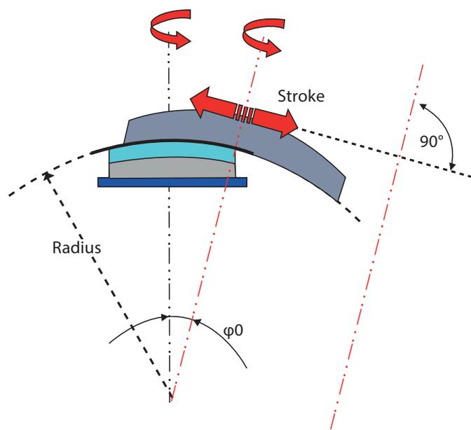
Figure 1: Theoretical kinematic model of tangential polishing process
