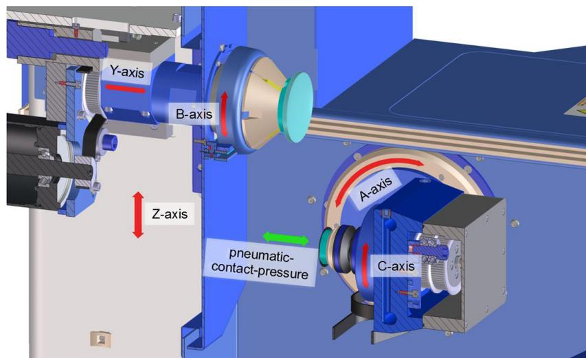
Figure 2: The configuration of axes in the Duo-FLEX polisher was designed for the tangential polishing process with static kinematics
