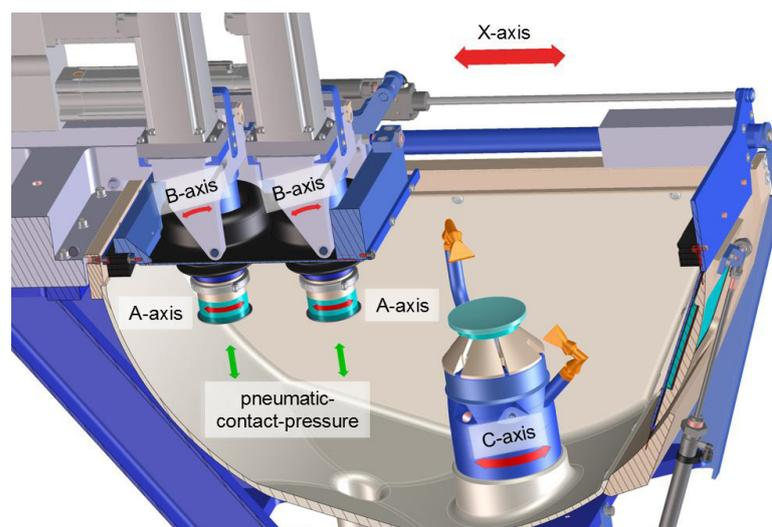
Figure 3: The advanced configuration of axes in the Multi-FLEX polisher is designed for the tangential polishing process with dynamic kinematics
