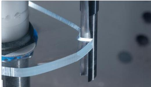
Dry-cut edgers are frequently 4 or 5 axes machines. Due to multiple axes, in conjunction with small tool diameters, dry cutting enables labs to cut shapes and special features (i.e. small radii, step bevel, etc.) formerly not possible to process with conventional edgers.
