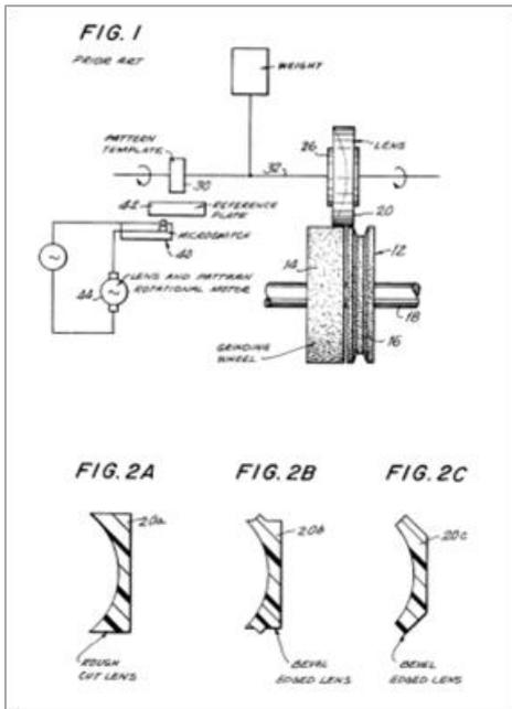
Edging began with ceramic wheels, then moved to diamond wheels. The principal edging technology is based on grinding, which generates heat on the lens surface. Because of this, water or a coolant is used to keep the wheels and work piece cool.
