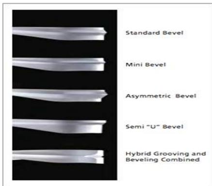
Tools are configured and exchanged based on specific features, i.e.: mini bevel, small radii, t-bevel, etc.
