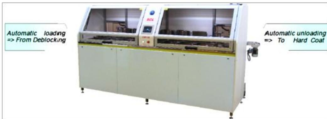
Picture 12: Automated lens cleaning machine CHP150
