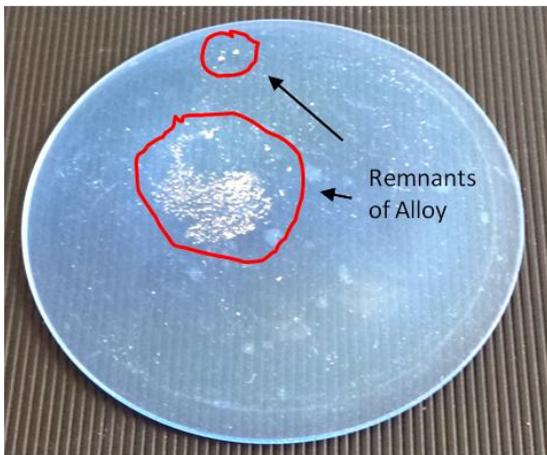
Picture 5: Alloy Residue on Protective Tape
