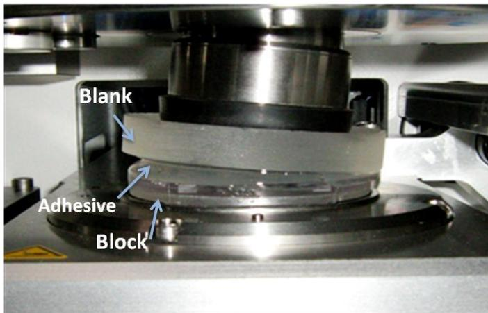
Because of the UV-glue's strong adhesive properties, the manual deblocking procedure used for alloy (hitting the blocked lens using a deblocking ring on a rigid surface) does not work. It is also not desirable due to the potential for lens breakage. Consequently it was necessary to develop a new deblocking process, referred to as water-jet deblocking.
