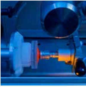
High-pressure water jet for lens deblocking.
