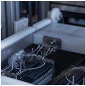
Chainless lens transfer system prevents chamber cross-contamination
